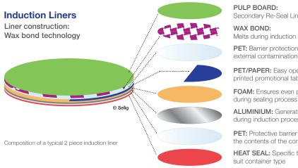
PULP BOARD: Secondary Re-Seal Liner WAX BOND: Melts during induction process PET: Barrier protection from
