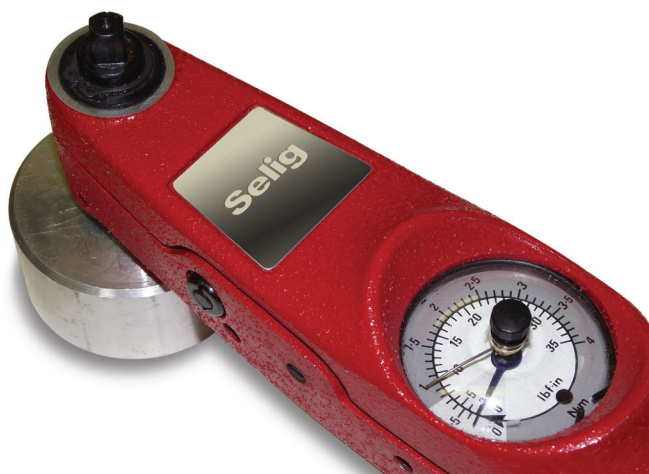
Figure 3a: The pressure is measured in Inch pounds or Newton Metres on a torque meter
